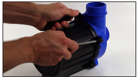
Step 4: Unscrew all four screws around the blue plastic impeller housing.
