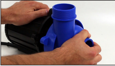
Step 7: Carefully pull away the impeller housing.
